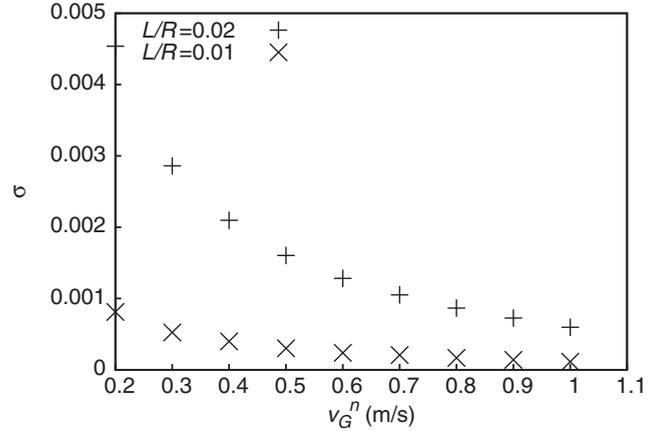
FIG. 6. Standard deviation of the fluctuating coefficient of restitution as a function of the normal component of the impact velocity. The eccentricity,  $L/R = 0.01$  and  $L/R = 0.02$ , corresponds to average quality glass spheres [19].
