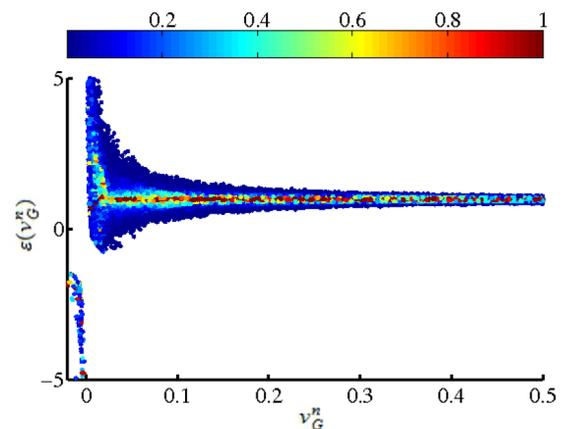
FIG. 7. (Color online) Same data as Fig. 2 but for smaller values of the argument. We observe  $\varepsilon < 0$  for low impact velocity. There are two different mechanisms leading to negative values of the coefficient of restitution corresponding to the two groups of data points appearing in the figure (for discussion see the text).
