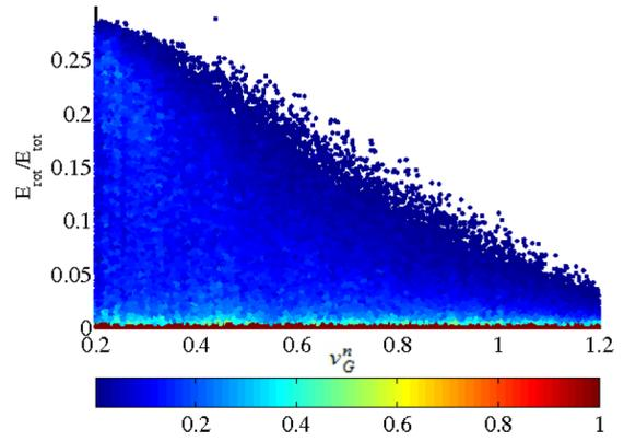
FIG. 3. (Color online) Ratio of rotational versus total energy, Eq. (12), as a function of the impact velocity,  $v_G^n$ . The data are colored according to the normalized frequency of occurrence.
