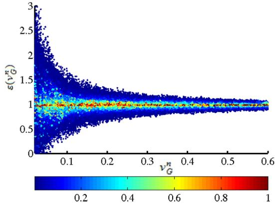
FIG. 2. (Color online) The macroscopic coefficient of restitution,  $\epsilon$ , versus the impact velocity,  $v_G^n$ , for eccentricity  $L/R = 0.1$ . The graph shows an abundance of 400 000 impacts. The data points are colored according to the normalized frequency of occurrence (see text for explanation).
