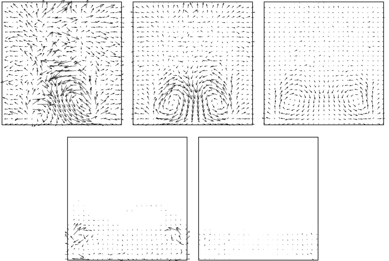
**Figure 2.** Images of the cycle-averaged motion of the system vibrated at  $f = 20$  for different velocities of forcing,  $A\omega$ : a) 1900, b) 1250, c) 600, d) 100, e) 15.
