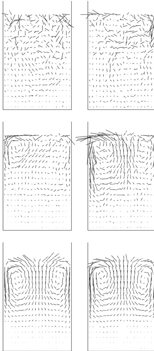
Fig. 1. – Convection rolls in systems without (left) and with the larger particle (right) for three different shaking frequencies,  $f = 2.6 \text{ sec}^{-1}$  (upper figure),  $f = 2.8 \text{ sec}^{-1}$  (central figure) and  $f = 3 \text{ sec}^{-1}$  (lower figure). In the central case the big particle triggers convection rolls. The pictures were obtained by averaging over 50 shaking periods of the box.
