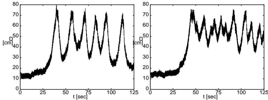
Fig. 4. – Evolution of the vertical position of the big particle as function of time, (a)  $\mathcal{R} = 2.0$  and (b)  $\mathcal{R} = 3.0$  for  $f = 3.2 \text{ sec}^{-1}$ .
