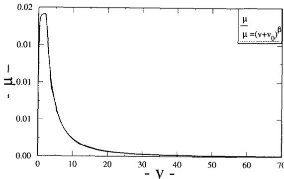
Fig. 4. Friction coefficient  $\mu$  as a function of  $v$ , homogeneously averaged over  $\alpha$ -values that range from  $0.2^\circ$  to  $2.0^\circ$ . Superposed we see the function  $\mu = (v + v_0)^\beta$  with  $v_0 = 3.308$  and  $\beta = -2.342$  fitted for  $2.2 \leq v \leq 70$ .
