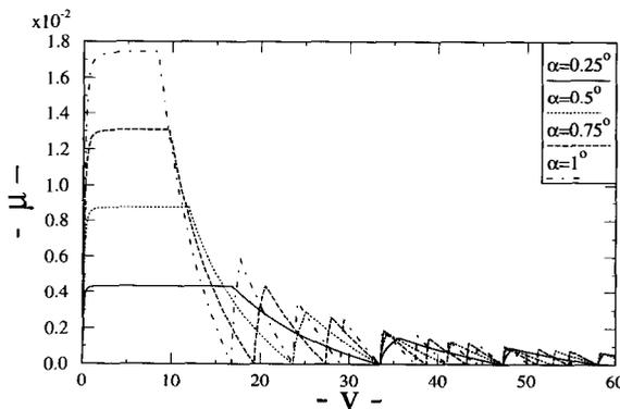
Fig. 3. Friction coefficient  $\mu$  as a function of the driving velocity  $v$  for different angles  $\alpha$  and  $B = 0.0035/\tan(\alpha)$ . We always use  $g = 9.81$ .
