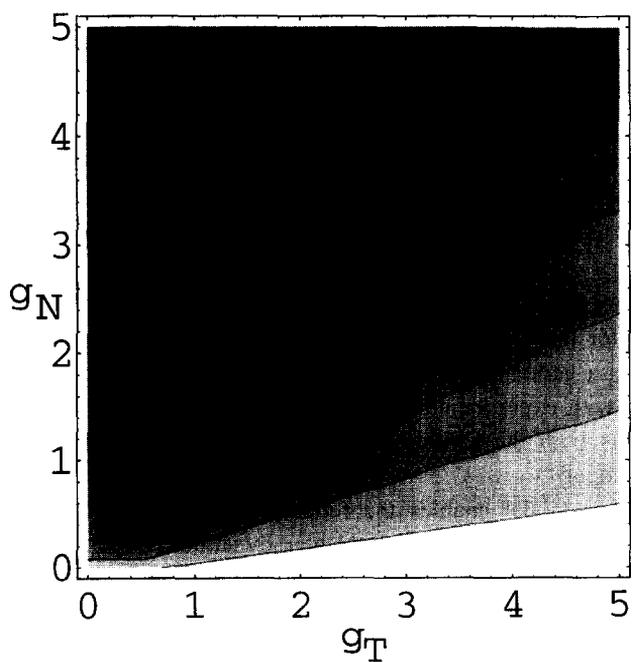
Fig. 3. The tangential restitution coefficient  $\varepsilon_T$  as function of the impact velocities  $g_N$  and  $g_T$  for two values of the surface roughness: (top)  $\zeta_0 = 10^{-7}R^{\text{eff}}$ , (bottom)  $\zeta_0 = 2 \times 10^{-4}R^{\text{eff}}$ .
