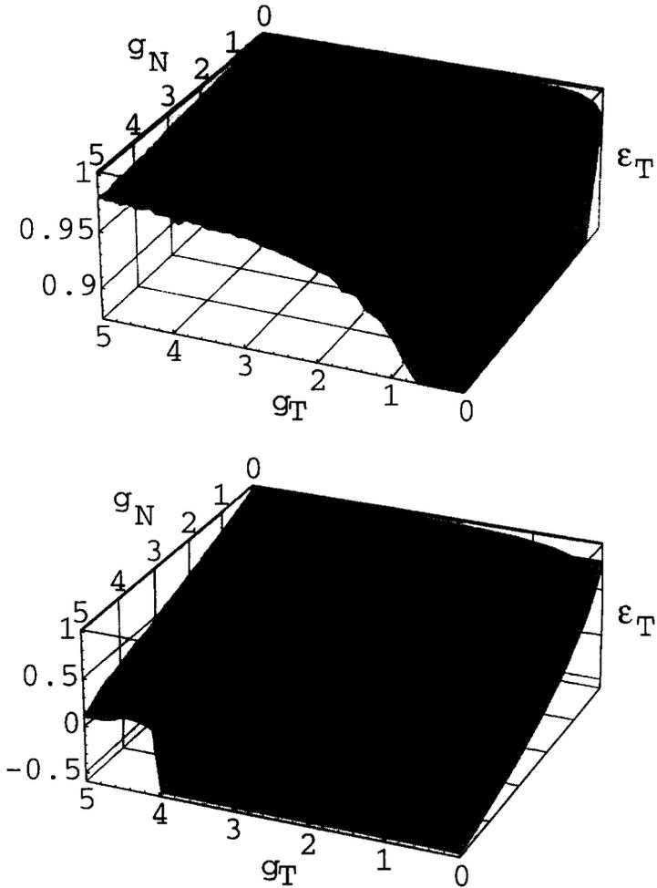
Fig. 4. Surface plot of the tangential restitution coefficient  $\epsilon_T$  versus the plane  $g_N$ – $g_T$  of the impact velocities for two values of the surface roughness (same values as in Fig. 3).
