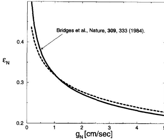
Fig. 2. The theoretical results for the normal restitution coefficient  $\epsilon_N$  as a function of the normal component of the impact velocity  $g_N$  agree with the experimental results [7] (dashed line).
