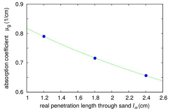
Figure 3: Attenuation coefficient  $\mu_g(l_g)$  obtained from the calibration measurements (symbols). The abscissa shows values of  $l_g = l_{\text{box}} \varphi$ , where  $l_{\text{box}} = \{2, 3, 4\}$  cm and  $\varphi = 0.6$ . The dashed line shows Eq. (4) using the calibrated parameters.
