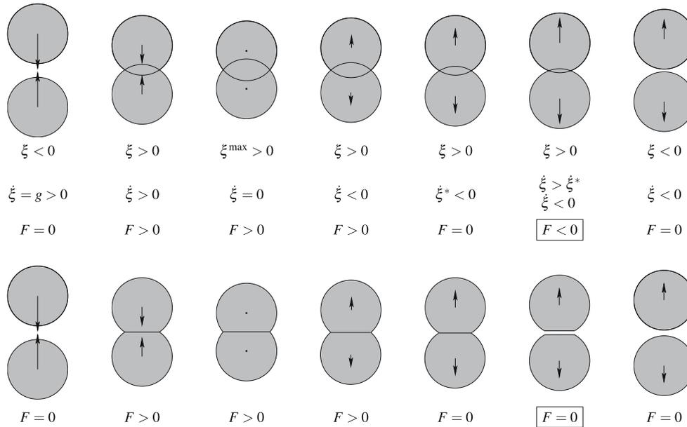
**Fig. 1** Sketch of a particle collision. The *upper part* of the figure visualizes the condition (16) for the end of the collision. As an artifact of the model, there appear attracting forces towards the end of the collision (*boxed notation*). *Lower part* the condition (19) for the end of the collision avoids this artifact
