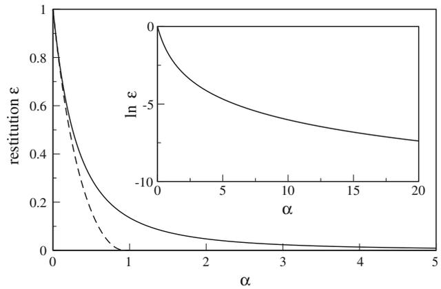
**Fig. 2** Coefficient of restitution as a function of  $\alpha \equiv \beta/\omega_0$ . The *dashed curve* is the result for the termination condition  $\xi(t_c^0) = 0$ . Obviously, for high damping  $\alpha > 1$  we have dissipative capture. The *full line* and the *inlay* show  $\varepsilon$  as a function of  $\alpha$  for the termination condition  $F(t_c) = 0$ . There is no dissipative capture even for very high damping
