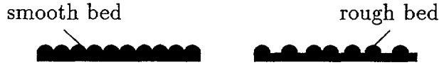
Fig.2. — Rough and smooth beds both consist out of spheres with diameter R_S = 0.66 \cdot R . In the case of the smooth bed these spheres are arranged close together while in the case of the rough bed they are arranged irregularly.
