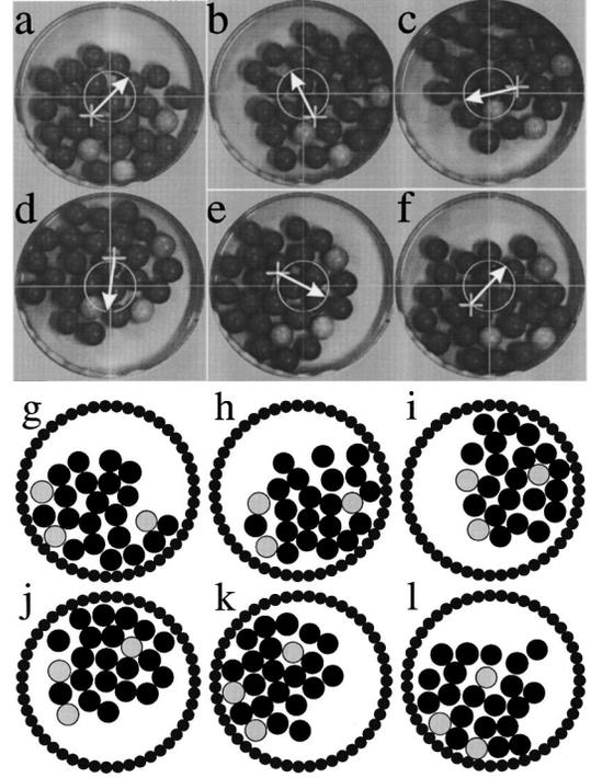
FIG. 2. Temporal behavior of a system of 26 spheres during one counterclockwise cycle of the swirl. The arrow shows the direction of the momentary acceleration. The lower six figures show the corresponding molecular dynamics simulation.
