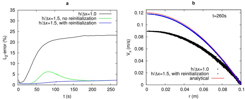
**Fig. 9.** (Color online) SPH simulation of pipe flow driven by a constant body force at  $Re = 120$ . (a) Evolution of the  $L_2$  error with and without density re-initialization for  $h/\Delta x = \{1, 1.5\}$ ; (b) velocity profile at time  $t = 260$  s obtained from SPH simulation in comparison with the analytical result [22]. The symbols show the streamwise velocity of all SPH particles versus their position in the direction normal to the wall.
