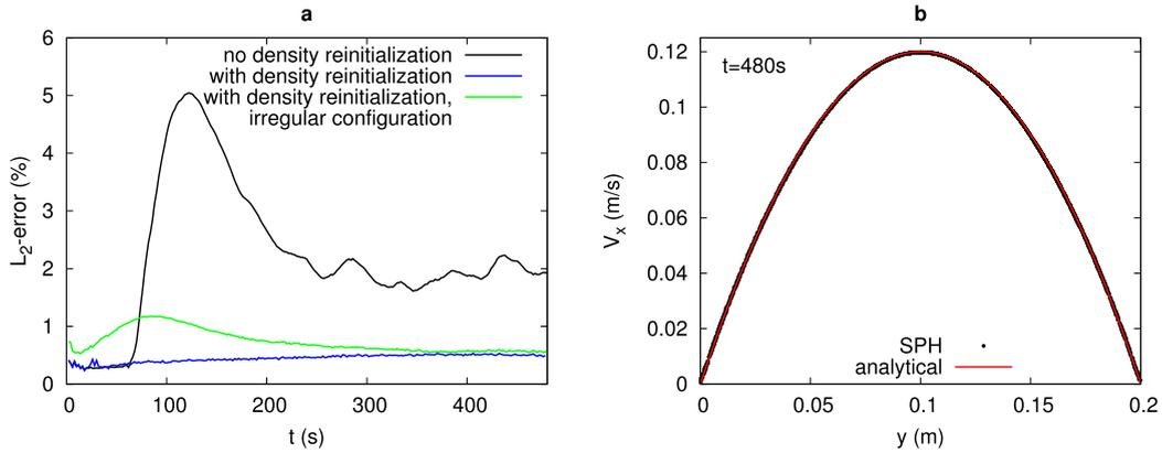
**Fig. 7.** Simulation results for Poiseuille flow ( $Re = 120, h/H = 0.02, h/\Delta x = 1.5$ ). (a) Evolution of the  $L_2$  error with and without density re-initialization. (b) Velocity profiles at  $t = 480$  s obtained from SPH with density re-initialization in comparison with the analytical solution. The symbols show the streamwise velocity of all SPH particles versus their position in the direction normal to the wall.
