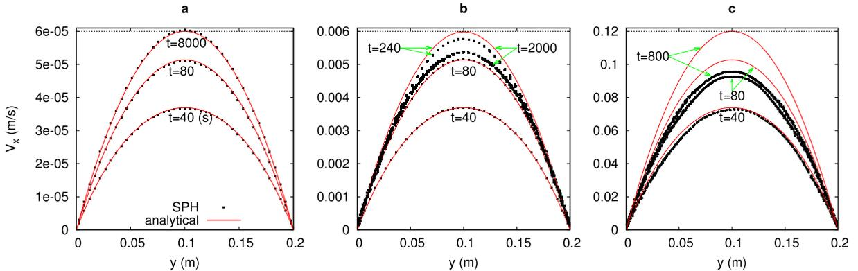
**Fig. 1.** Failure of SPH in transient plane Poiseuille flow. Velocity profiles of plane Poiseuille flow for (a)  $Re = 0.06$ , (b)  $Re = 6$ , and (c)  $Re = 120$  at different time,  $t$ , starting at rest at  $t = 0$ . The symbols show the streamwise velocity of all SPH particles versus their position in the direction normal to the wall. The lines show the analytical solution [22].
