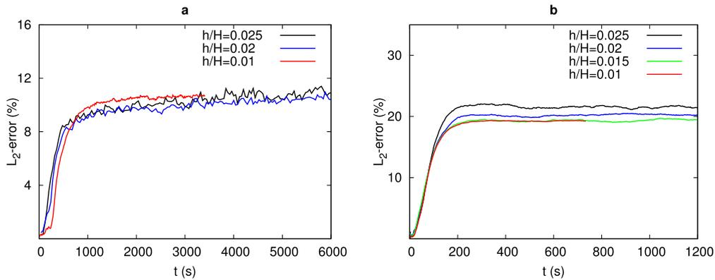
Fig. 2. Evolution of the  $L_2$  error given by Eq. (13) for different smoothing lengths,  $h$ . (a) Poiseuille flow at  $Re = 6$ ; (b) at  $Re = 120$ .
