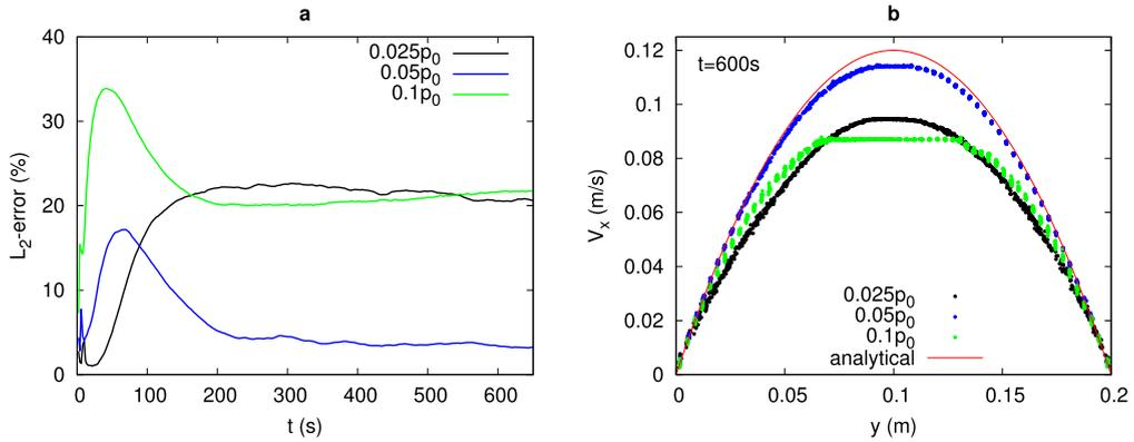
**Fig. 3.** (Color online) Simulation results for Poiseuille flow ( $Re = 120$ ,  $h/H = 0.02$ ,  $h/\Delta x = 1$ ) at different background pressure values,  $0.025 p_0$  (black),  $0.05 p_0$  (blue), and  $0.1 p_0$  (green). (a) Evolution of the  $L_2$  error; (b) velocity profiles at  $t = 600$  s. The symbols show the streamwise velocity of all SPH particles versus their position in the direction normal to the wall. Lines show analytical solutions.
