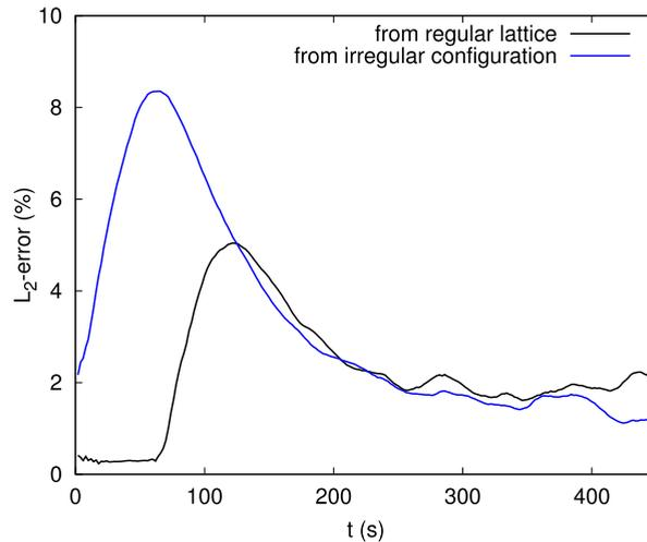
Fig. 5. Evolution of the  $L_2$  error given by Eq. (13) for Poiseuille flow at  $Re = 120$  ( $h/H = 0.02$  and  $h/\Delta x = 1.5$ ) with different initial particle settings.
