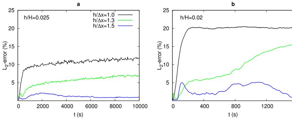
**Fig. 4.** Evolution of the  $L_2$  error given by Eq. (13) for different ratios of smoothing lengths to particle spacing,  $h/\Delta x$ . (a) Poiseuille flow at  $Re = 6$ ; (b) at  $Re = 120$ .
