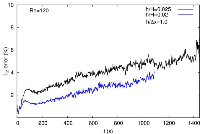
Fig. 6. Evolution of the  $L_2$  error for Poiseuille flow ( $Re = 120$ ,  $h/H = 0.025$  and  $0.02$  with  $h/\Delta x = 1.0$ ) using the density re-initialization technique.
