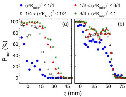
FIG. 5. Number fraction  $P_{\text{out}}$  of particles that were at the outer volume of the tube at  $t = 0$ .  $P_{\text{out}}$  is shown as a function of the vertical position  $z$  for different values of the radial position  $r$ . (a) and (b) refer to simulation results at  $t = 10T$  and  $t = 75T$ , which correspond to snapshots in the ascending and steady-state regimes, respectively.
