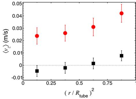
FIG. 4. Average vertical velocity  $\langle v_z \rangle$  of the particles in the tube as a function of the squared nondimensional radial position,  $(r/R_{\text{tube}})^2$ . Circles denote results for the ascending phase ( $t \lesssim 20T$ ), while squares correspond to the steady-state phase ( $t \gtrsim 50T$ ). The dotted line indicates  $\langle v_z \rangle = 0$ .
