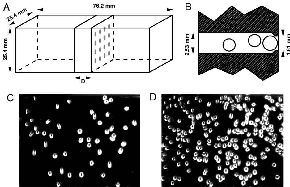
**Fig. 3.** The experimental system and pictures of the granular gas. (A) Diagram of the experimental setup. (B) Cross-section of a circular pore that has a reduced diameter on the right end, too small for the larger particles in the binary mixture to pass. (C) Side view image of 50 beads in a chamber. (D) Side view image of 250 beads in a chamber.
