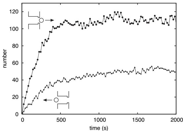
**Fig. 5.** Number of beads measured to pass through a membrane (9.53 mm thick), as a function of time, when only small beads were present. Flow in the direction from the large to the small end of the pores is enhanced relative to that for the reverse orientation of the pores. There was a total of 200 beads; those residing in the pores were not observed.
