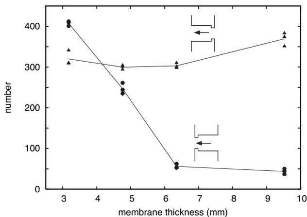
**Fig. 4.** Number of small beads measured to cross the membrane after 3 min, as a function of membrane thickness, for the two flow directions (cf. Fig. 3). The loaded side of the membrane initially had a mixture of 1,600 small beads and 400 large beads.
