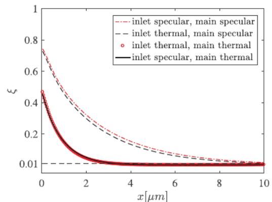
Fig. 2. Effect of wall characteristics of a T-shape micromixer. Degree of mixing,  $\xi$ , (see Eq. (1)) as a function of the downstream position along the main channel,  $x$ , for the combinations of boundary conditions.
