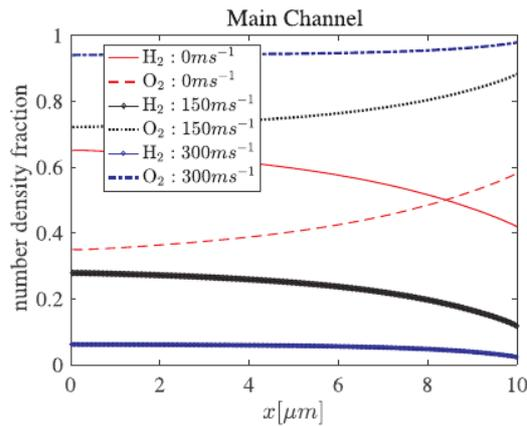
Fig. 7. Number density fraction of  $H_2$  and  $O_2$  as a function of the downstream position in the main channel for various values of the inflow velocity.
