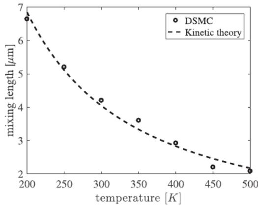
Fig. 4. Influence of temperature on the mixing length. DSMC simulation (circles) and kinetic theory (dashed line) according to Eq. (8) with  $\alpha = 0.809$ ,  $\beta = 0.235$ .
