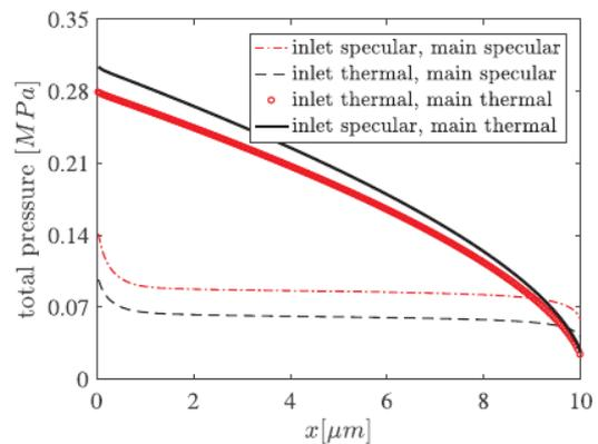
Fig. 3. Comparison of average pressure drop in the main part of T-mixer.
