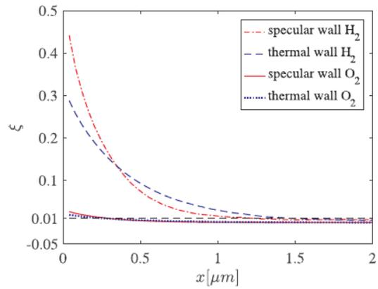
Fig. 6. Effect of wall characteristics (specular and thermal) of a T-shape micromixer on gases with different molecular mass. Degree of mixing,  $\xi$ , (see Eq. (1)) as a function of the downstream position along the main channel,  $x$ .
