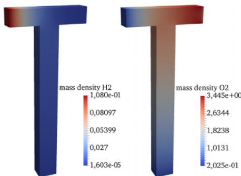
Fig. 8. Mass density of  $H_2$  and  $O_2$  in a T-shape micromixer with an inflow velocity of  $300\text{ms}^{-1}$ .
