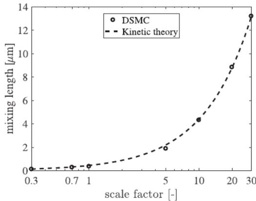
Fig. 5. Mixing length as a function of the scaling factor. Points: DSMC simulation results for  $v = 50 \frac{\text{m}}{\text{s}}$ ; line: prediction from kinetic theory, Eq. (8).
