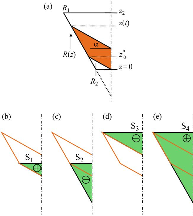
FIG. 7: (a) Sketch of the sub-volume III (orange) to introduce the nomenclature. (b-e) Segments of volumes of positive  $\oplus$  and negative  $\ominus$  masses used in the calculation. Their superposition results in volume III.
