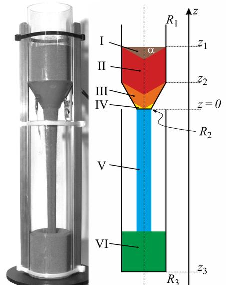
FIG. 2: Experimental setup (left). The sketch (right) introduces the geometric parameters and defines the sub-volumina I – VI where  $\alpha$  is the angle of repose. The sketch shows a cut through the symmetry axis.
