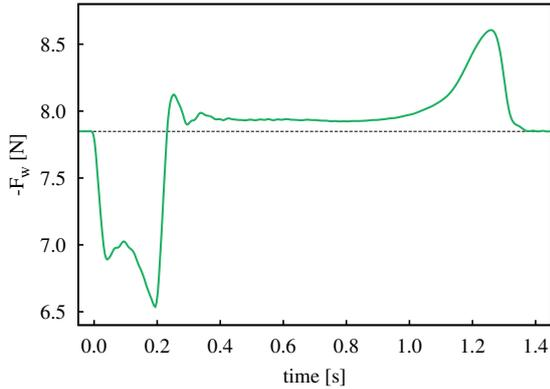
FIG. 3: Weight of the granulate inside the hourglass as a function of time (the weight of the apparatus subtracted). At time  $t = 0$  the orifice opens. We observe a characteristic evolution which can be understood in detail from the theory presented in Sec. III.
