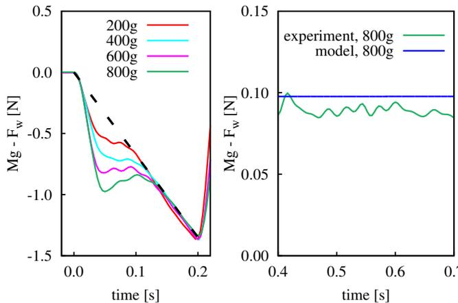
FIG. 14: Left: Experimentally measured weight in the initial interval  $t < 0.22$  s for different amounts of granular material (magnification of Fig. 13). The figure illustrates the appearance of the initial negative peak due to the acceleration of the total amount of granular material after opening the lid at  $t = 0$ . Right: Magnification of the plateau in Fig. 13. The deviation of the experimental and theoretical result is about 10%.
