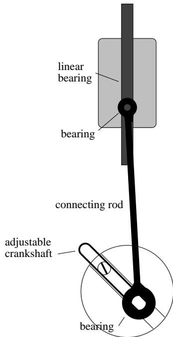
**Fig. 2.** The framework which holds the column of spheres was mounted on a linear bearing and was driven via a crankshaft.
