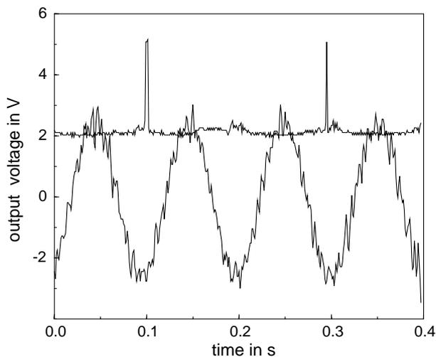
**Fig. 11.** The output of the acceleration sensor (lower curve). One can see that the sinusoidal curve of the driving frequency is disturbed by higher frequency oscillations. The higher frequencies account for up to 20% of the maximum acceleration. The upper curve shows the conductivity measurement of the topmost beads. The peaks correspond to jumping of the topmost bead.
