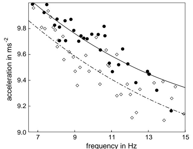
**Fig. 10.** All relevant data points together with a least-squares fit curve according to template equation (8). Full circles: 2 beads, diamonds: 20 beads.
