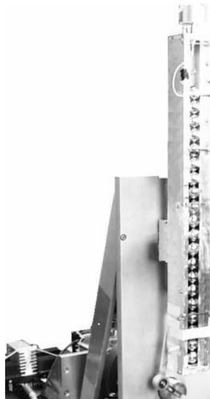
**Fig. 4.** Experimental device with column of steel spheres.
