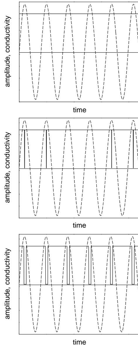
**Fig. 6.** For subcritical shaking the particles are always in contact, *i.e.*, the conductivity (solid line) is constant (top). For over-critical shaking the conductivity drops to zero in each period (bottom). For critical values the conductivity shows irregular peaks (middle).
