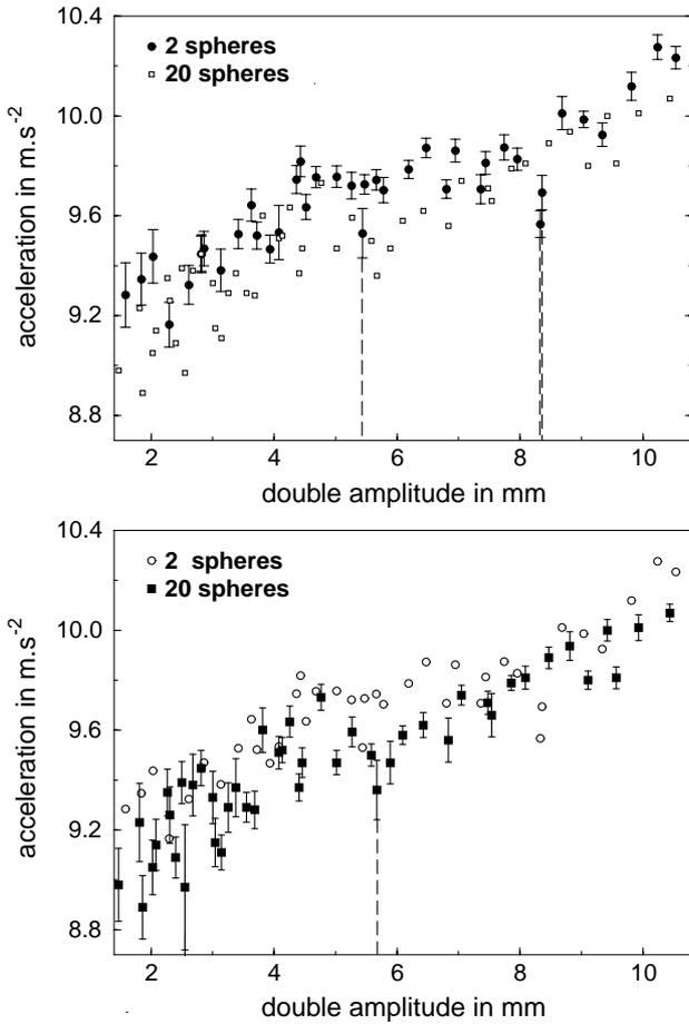
**Fig. 7.** All measured data points. In the upper figure error bars have been attached to the measurement for a single free-moving bead (and another one serving as a well-defined lower boundary). In the lower part the same data is shown with error bars for the measurement using 20 spheres. Data points marked by dashed lines have been disregarded for further analysis since they are adulterated by resonances of the equipment (see text).
