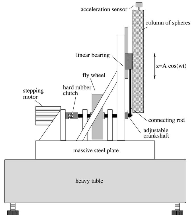
**Fig. 3.** Sketch of the experimental device.
