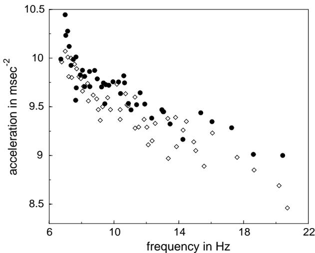
**Fig. 8.** The critical acceleration *vs.* frequency. Circles represent data of two spheres (reference), diamonds represent data for 20 spheres.
