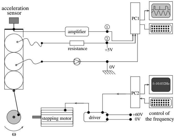
**Fig. 5.** The onset of fluidization was determined by observing interruptions of the electrical circuit.
