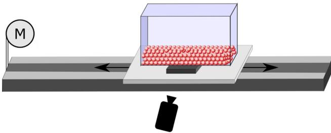
FIG. 1. Sketch of the experimental setup. A rectangular container is partly filled with monodisperse steel spheres and mounted on a sledge. The sledge is harmonically driven by a step motor with a frequency of 3 Hz, while the amplitude is varied to change the acceleration. The dynamics of the spheres is monitored by a camera from the front. In most of the measurements the diameter of the spheres is 4 mm.
