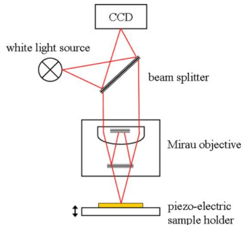
FIG. 3. (Color online) Principle of operation of a vertical scanning interferometric microscope.
