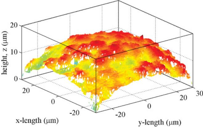
FIG. 4. (Color online) Height map of the cap of a large Mo-Sci grain etched for 4 min.
