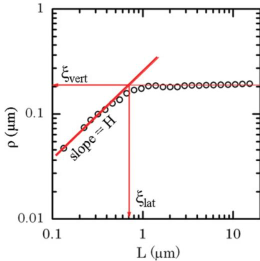
FIG. 6. (Color online) The roughness,  $\rho(L)$ , on a double logarithmic scale, yields the vertical and lateral saturation length scales,  $\xi_{\text{vert}}$  and  $\xi_{\text{lat}}$ , here for a Cataphote grain etched for 30 s. The slope of the fit through the first five data points is the Hurst exponent  $H$ .
