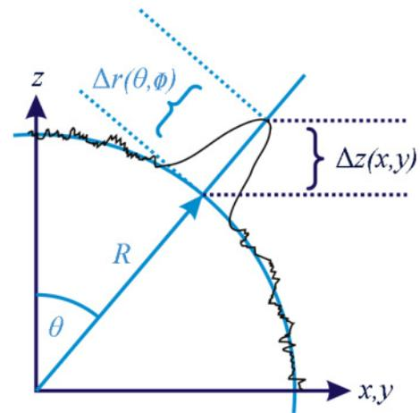
FIG. 13. (Color online) When analyzing the roughness of the glass spheres, we need to make an angle-of-sight correction to account for our having measured height in the  $z$  coordinate instead of in the radial direction.  $R$  is the sphere radius, and  $\Delta z(x, y) = h(\theta, \phi)$  is the height of the grain profile measured vertically from above. The correct radial height of the feature is given by  $\Delta r = \frac{\Delta z}{\cos \theta}$ .
