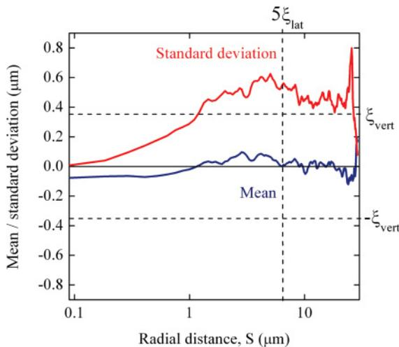
FIG. 15. (Color online) Radial average and standard deviation of a different large Mo-Sci grain etched for 1 min. This grain is rejected: the standard deviation exceeds the range  $[-\xi_{\text{vert}} \dots \xi_{\text{vert}}]$  for  $L < 5\xi_{\text{lat}}$ .
