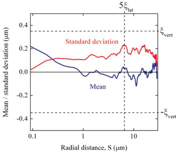
FIG. 14. (Color online) Radial average and standard deviation of a large Mo-Sci grain etched for one minute. This grain is accepted: both lines remain within the range  $[-\xi_{\text{vert}} \dots \xi_{\text{vert}}]$  for  $L < 5\xi_{\text{lat}}$ .
