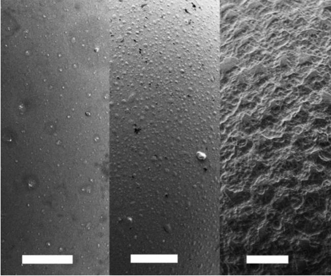
FIG. 1. Scanning electron microscope images of the surfaces of MoSci glass spheres of diameter  $146 \pm 19 \mu\text{m}$  (small Mo-Sci). Left: Smoothed by NaOH. Center: Untreated. Right: Etched for 4 min. The white bars are  $10 \mu\text{m}$  long.
